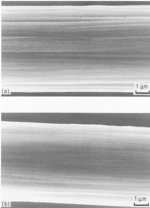
Figure 4 SEM photographs of (a) uncoated and (b) PVAL-coated carbon fibres.
