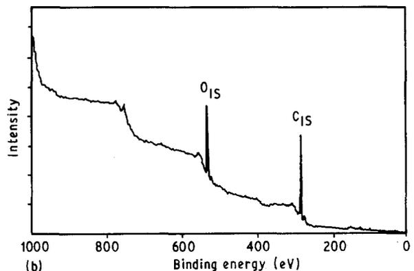
Figure 1 X-ray photoelectron survey spectra of (a) uncoated and (b) PVAL-coated carbon fibres.
