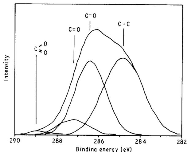
Figure 3 Gaussian peak fitting of the C1s spectrum of uncoated carbon fibres.
